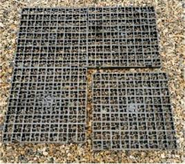
Interlocking square panels which are light and easy to handle. They are made from Recycled plastic. These must be laid before delivery of your building ideally on sand to ensure that they are level. The open nature of the base allows water to drain away naturally from your garden building whilst promoting air flow under your building, which reduces the chance of it becoming rotten. For larger buildings you may want to weigh this down by putting shingle within the base squares.
